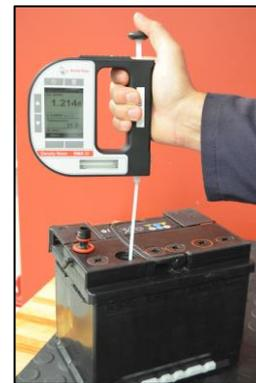
**Image 11: Acid density measurement of batteries**
