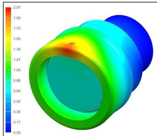
**Image 3 & 4: Finite element models of a press fit component**
