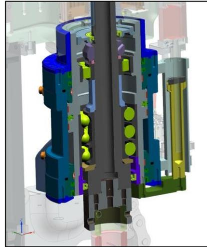
**Image 2: Cross-section of the WC4 Boss Welding Machine spindle arrangement**
