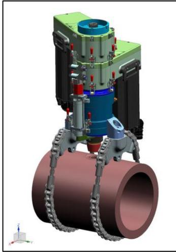
**Image 1: Design of the in-house commissioned WC4 Boss Welding Machine mounted on a modelled specimen**
