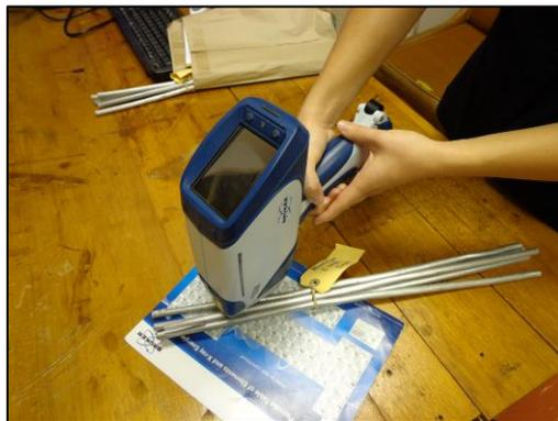
**Image 10: Elemental analysis using XRF**
