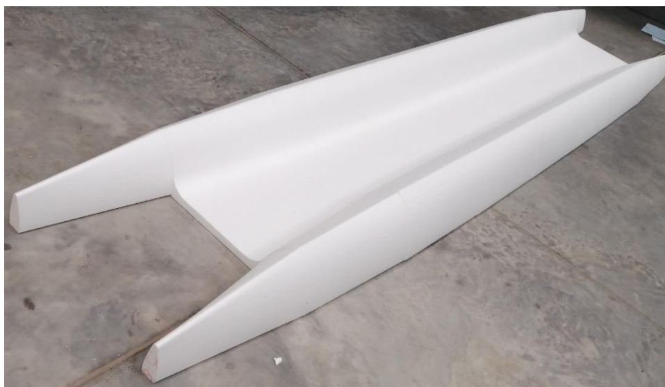
Figure 68: Prototype core cut using Hot-Wire foam cutter
