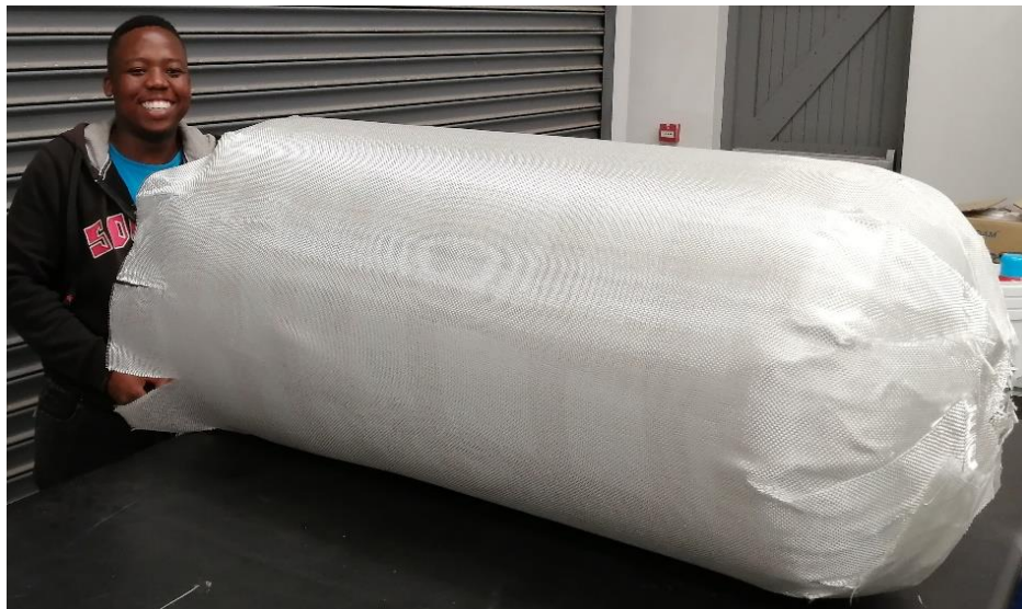
Figure 72: Prototype tank evaluation of manufacturing technique via vacuum infusion [Model tank container for shipping chemicals]
