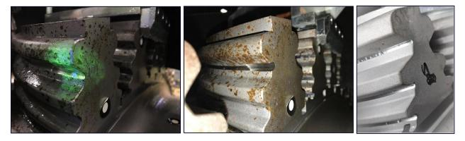
Images above: Before and after images of crack and serration post grinding
