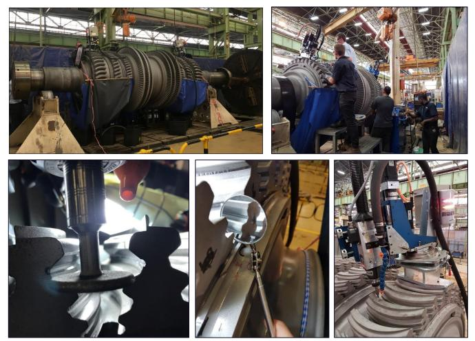
Top two images indicate the rotor and a team on site performing rotor serration grinding, the lower images are of the tools utilised and the completed grind
